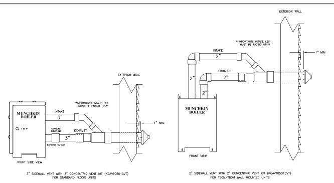
\*\*IMPORTANT NOTE: All vent pipes must be glued, properly supported and the exhaust must be pitched a minimum of a 1/4" per foot back to the heater (to allow drainage of condensate).
